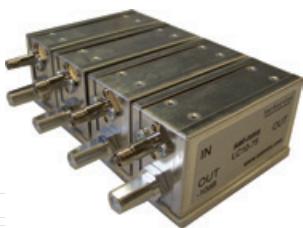
sat-nms LD10 L-Band Splitter
