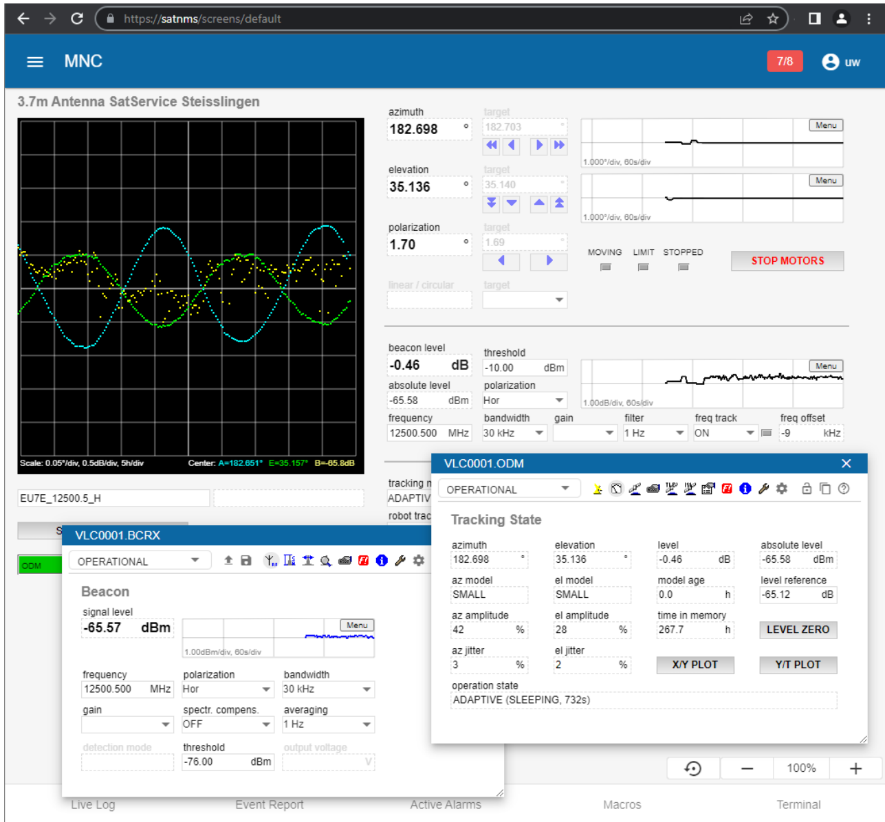
Figure 5: comprehensive screen for an antenna tracking system and ACU and beacon receiver device windows
