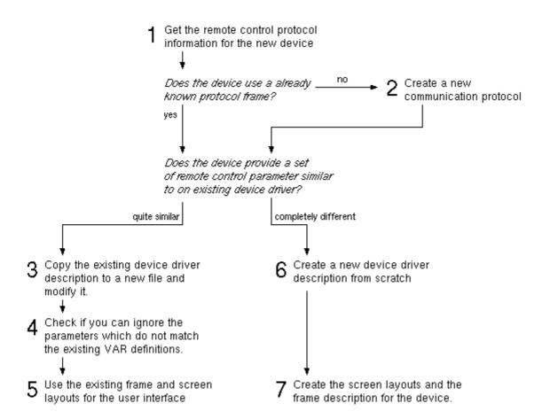
The diagram above illustrates the first steps to the integration of a new device type into the **sat-nms** software. You are encouraged to use as much as possible of the existing protocol, driver and user interface definitions.
